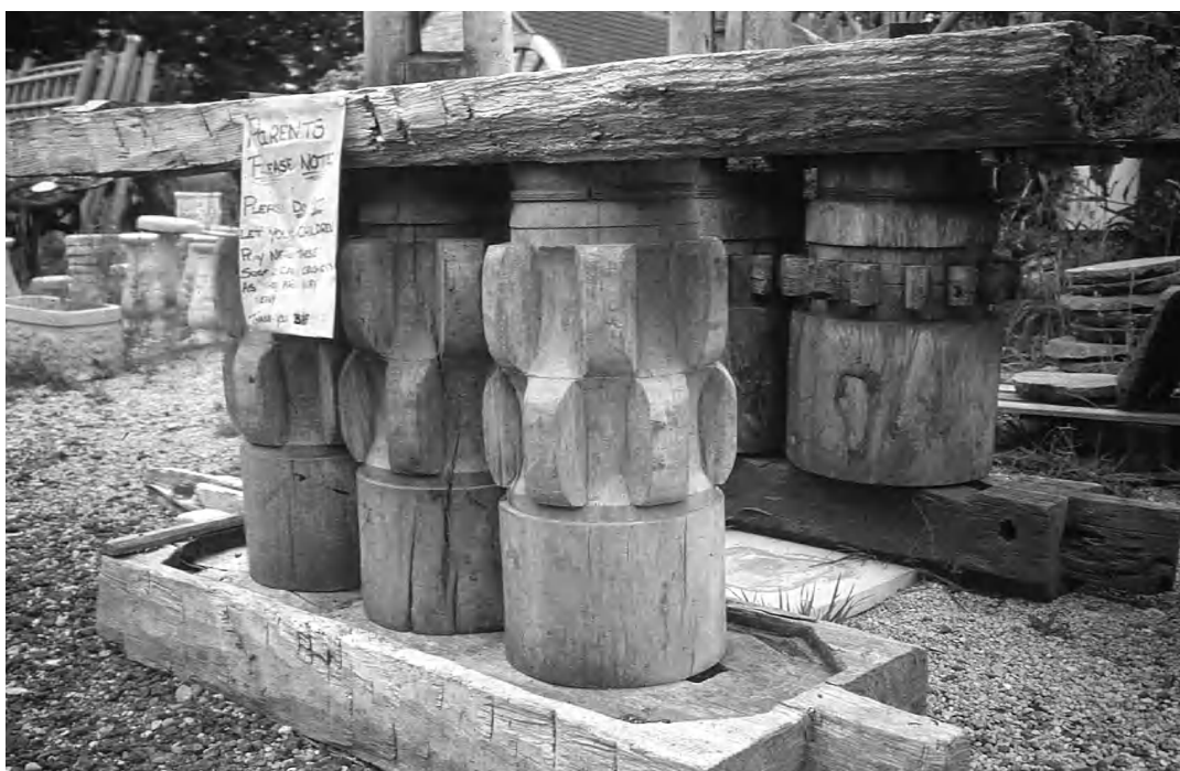
Fig. 6. Animal-powered sugar mills from Thailand; all parts are of wood including the rollers.
